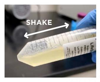
NOTE User should feel LifeSupport™ moving and hitting the cap and inner surfaces of the tube during shaking.
