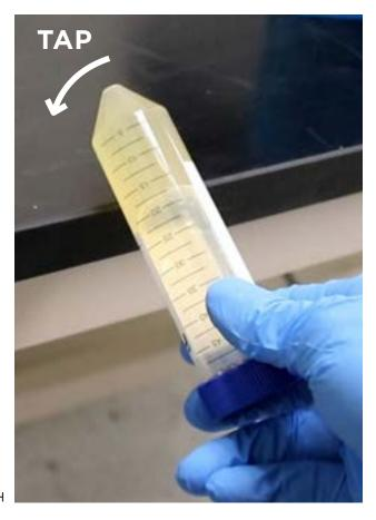
NOTE This is to dislodge the compacted LifeSupport™, allowing it to flow down towards the cap during tapping.
