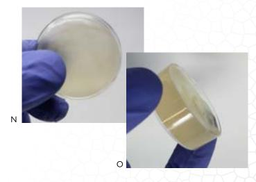
It is recommended that you use a print container that provides a minimum of 1 mm clearance on the bottom and a minimum of 3 mm clearance on all sides as well as the top of the construct to be printed. Additional clearance is fine, but requires using more LifeSupport™.
