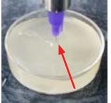
Unlike typical printing, the needle does not have to start out touching or even be close to the bottom of the container. The support bath will trap your print in place no matter where you start.
